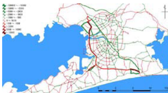
Simulated predictions of changes in traffic volume on roads in the vicinity of Toyohashi (Red: Increase, Green: Decrease)
