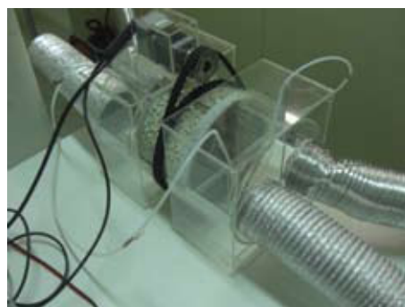
Fig.3 Air flow window based on adsorption/desorption effects
